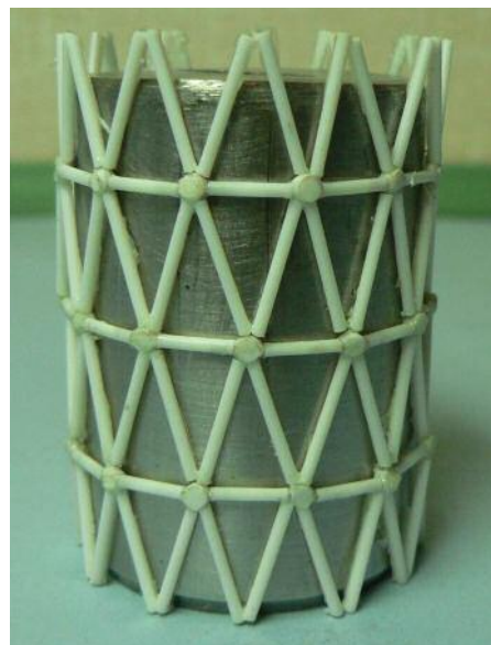
The lattice cage cylinders around a king pin.
