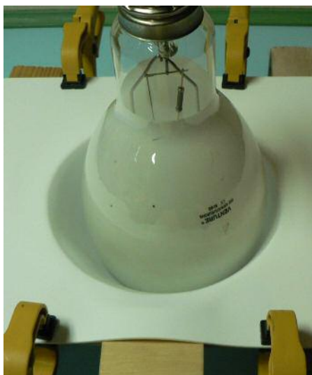
Plunge-moulding the internal fuel tanks.
